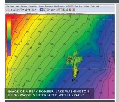
WASSP data is displayed in real-time, enabling you to make on the spot decisions. Instantly locate underwater debris or structures that might pose a hazard, and determine their precise size, shape and position.
